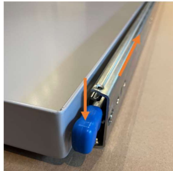
Figure 3. Push down on the blue lever, then slide the outer part of the drawer slide to remove it from the tray.
