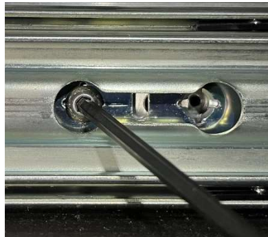
Figure 8. Tighten the M6 bolts with the supplied hex key, the front fixings are accessed through the middle section of the drawer slides.
