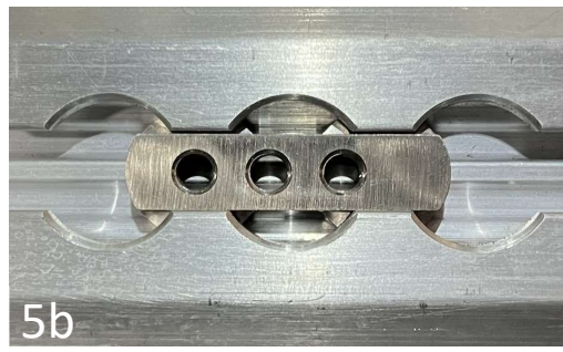
Figure 5a and 5b. Slide the nut so that the lobes are symmetrically aligned behind the teeth of the airline rail.
